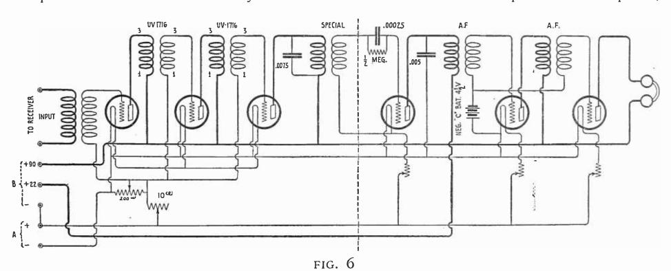
Intermediate-frequency amplifier with tuned output circuit. Material to the left of the dotted line is extra equipment necessary. Material on the right of the dotted line is the regular detector and two-stage audio-frequency amplifier
