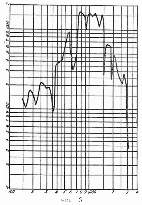
Showing the sound distribution for a loud speaker of the enclosed-armature type. The horizontal axis represents the frequency, from 100 to 10,000 cycles, and the vertical axis represents loudness
