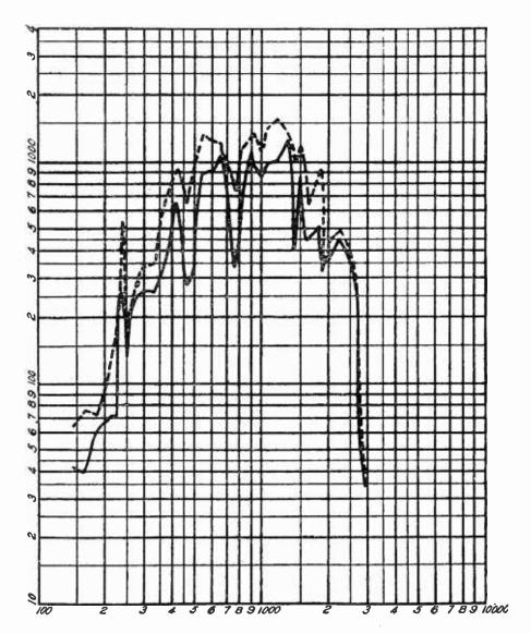
Two curves taken with the same relay-type loud speaker; in one case, the gap was .015 in. (solid line), and in the other, the gap was .010 in. (dotted line)
