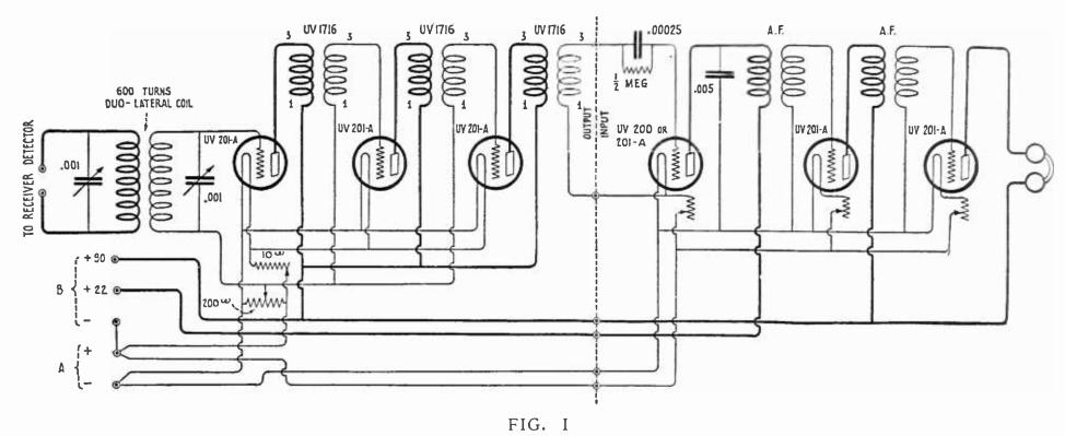
Additional material required for the construction of the intermediate amplifier of the super-heterodyne is shown to the left of the dotted line. Material to the right of the dotted line is the conventional detector and two-stage audio-frequency amplifier, details of which have appeared in past issues of Radio Broadcast. This type of intermediate amplifier is tuned at the *input* to the amplifier by the 600-turn DL coils, shunted by .001 mfd. variable condensers
