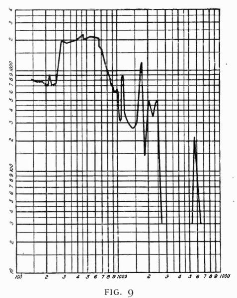
Showing the variation of sound intensity (vertical axis) with frequency (horizontal axis) when a small stiff diaphragm is used
