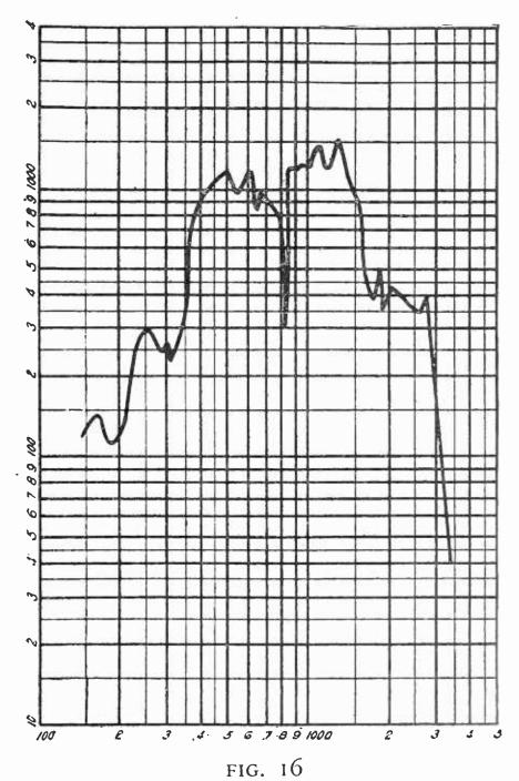
In this case the armature was not stiff enough and the sound showed a reduction in volume at 800 cycles
