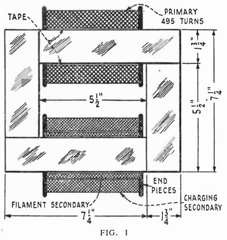
Showing how the core is built up of iron strips and how the two windings are placed. The primary and secondary windings are shown cut away on the side nearest the observer, so as to show the iron core over which the turns of wire are actually made
