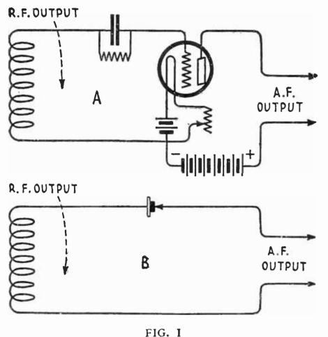
The fundamental circuits for bulb and crystal detection
