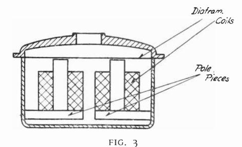
Loud speaker unit operated on the same principle as the ordinary telephone receiver
