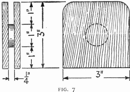
This special transformer is used as indicated in Fig. 6 (marked "special"). The walls of this transformer may be made of bakelite or hard rubber. The primary is wound with 200 turns of No. 29 S. C. C. and is separated from the secondary, which has 1500 turns of No. 36 D. S. C., by several layers of empire cloth
