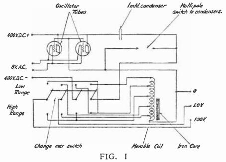
Oscillator designed to cover a range from 150 to 10,000 cycles
