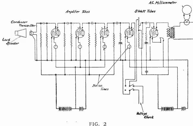
Apparatus for measuring the sound from a loud speaker
