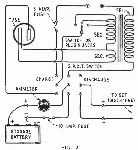
Diagram showing how to connect the transformer to the bulb and panel apparatus shown in last month's Lab
