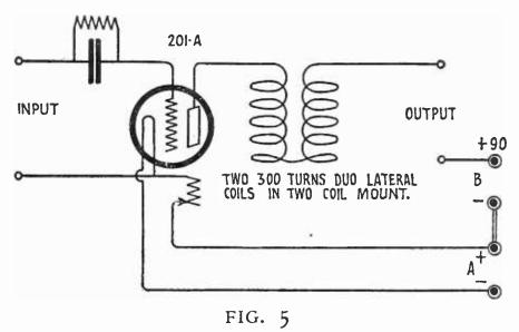
Connection to second detector of amplifier shown in Fig. 4, to permit reception of C. W. The two coils shown act as a variometer to tune the plate circuit of the second detector
